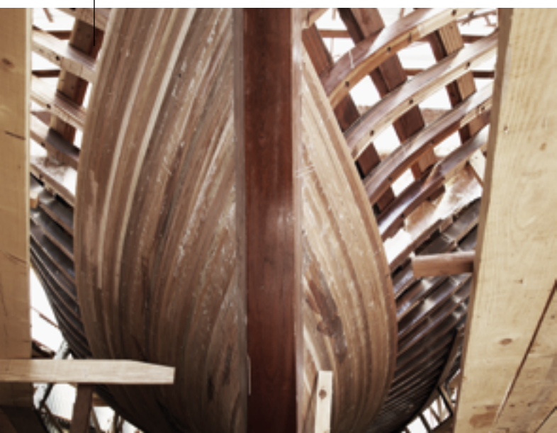
The skeleton of the gulet: the ribs
