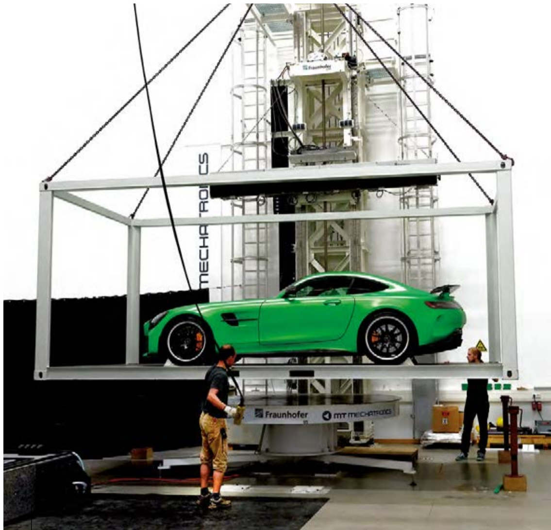
The lifting platform must be precisely oriented before the X-ray images are taken.
